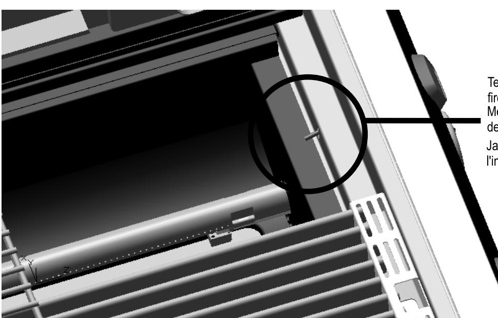
Temperature Gauge must be inside firebox
